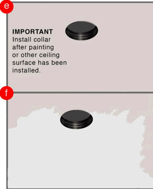
Step E/F- Flanged collar should be installed after painting, wood, metal ceiling has been prepped.
