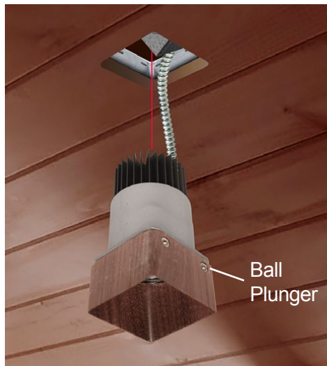
Step 5 - Ball plungers on lamp assembly click into metal flange in ceiling. If plungers are not secured to metal flange, lamp assembly might fallout.
